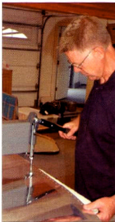
The EA DRDT-2 dimpler at hand, RV-10 builder John Ackerman dimples a rudder skin with peak rates of six dimples per minute.
