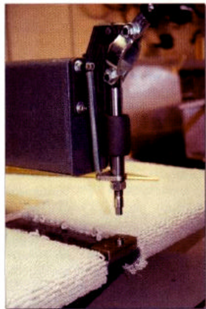
The business end of the EA dimpler. Note that the male dimple die is well above the plane of the table.
